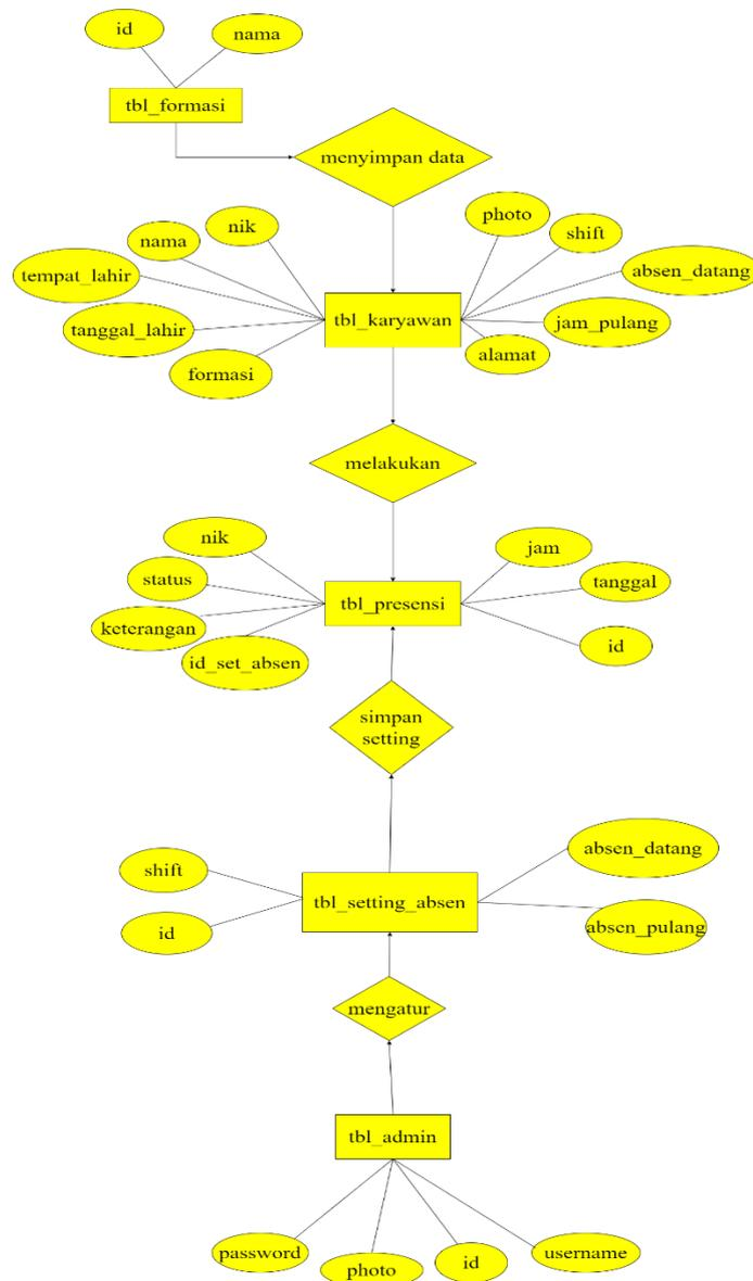
Gambar 3.1.7 Entity Relationship Diagram sistem presensi
