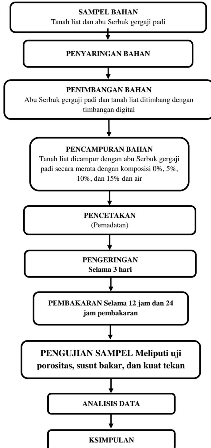
**Gambar 3. 2** Langkah-langkah prosedur penelitian
