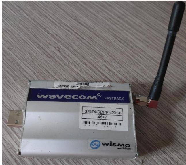
Gambar 3.6 Modem GSM
