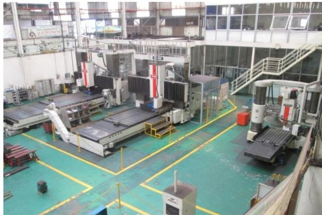
Gambar 2.20. Mesin *Machining Shin Nippon Koki 3 axis*
