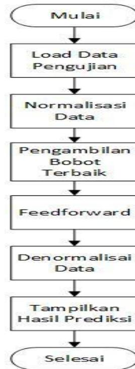
Gambar 3.4 Flowchart Pengujian JST (Dini, 2010)
